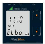
Enter New / Change Elbow value of the Output 1, second digit entered, prompting for third digit. (\*Denotes that digit will be flashing).
