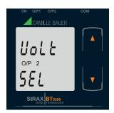
Pressing the " Down" key will enter the "output 2 type edit" mode and scroll between voltage and current.
