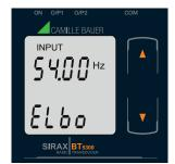
Pressing the " Down" key will enter the "New/Change Elbow value of the Input edit" mode.
