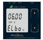
Pressing the " Down" key will enter the "New/Change Elbow value of the Output 2 edit" mode.
