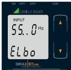
Enter New / Change Elbow value of the Input, second digit entered, prompting for third digit. (\*Denotes that digit will be flashing).
