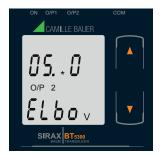
Enter New / Change Elbow value of the Output 2, second digit entered, prompting for third digit. (\*Denotes that digit will be flashing).
