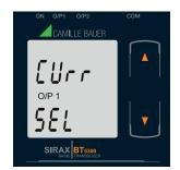
Pressing the " Down" key will enter the "output 1 type edit" mode and scroll between voltage and current.
