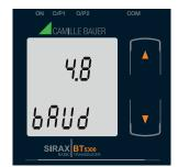
This screen allows the user to set Baud Rate of RS 485 port. The values displayed on screen are in kbaud.
