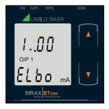
Enter New / Change Elbow value of the Output 1, first digit entered, prompting for second digit. (\*Denotes that digit will be flashing).
