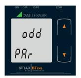
Pressing the " Down" key will enter the "Parity & stop bit edit" mode and scroll the value through odd: odd parity with one stop bit
