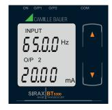
Screen 6: Voltage Input and Output 2 as Current
