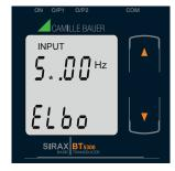
Enter New / Change Elbow value of the Input, first digit entered, prompting for second digit. (\*Denotes that digit will be flashing).
